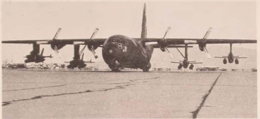
A DC-130A of Tactical Air Command's Combat Angel Force launches and controls 4 drones and multiple AQM-34Hs.
