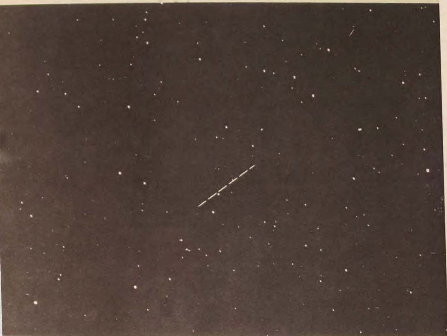
Film strip section from a Baker-Nunn camera shows the movement of a satellite in relation to stars.
